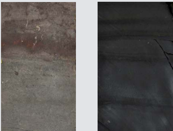
Figure 2. Examples of core from the Government Taylor A-1. The core from a depth of 7,948 ft. (left) has a strong reddish hue that suggests that organic matter in this rock has been oxidized. The total organic carbon (TOC) in this sample is only 0.21%, indicating poor source rock quality. The dark gray to black core from the depth of 7,977 ft. (right) is an excellent, thermally mature, source rock with a TOC of 11.25%, a hydrogen index of 669 and a T_{max} of 446°C. Width in photographs represent 3.25 inches of core.
